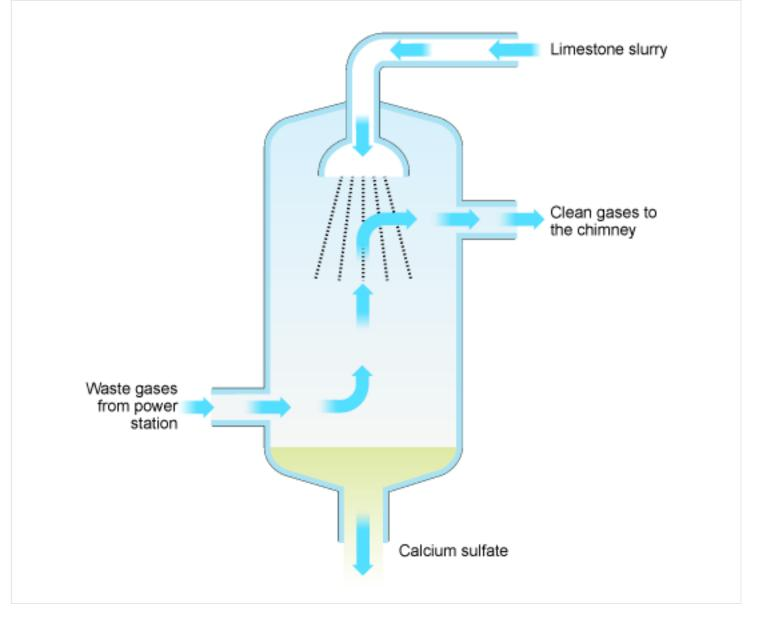
The process of removing sulfur dioxide
